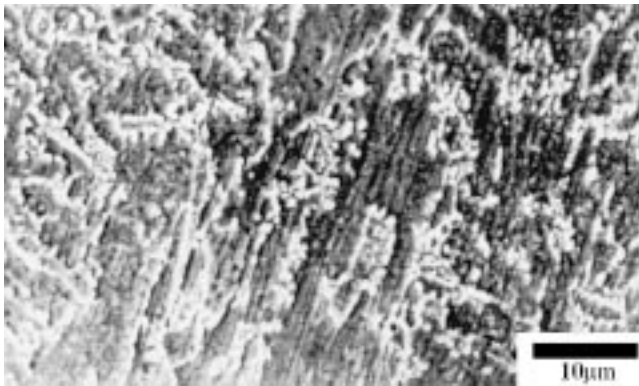
Fig. 10 Microstructure of the HAZ subjected to the heat treatment for 21.2 h. SEM
