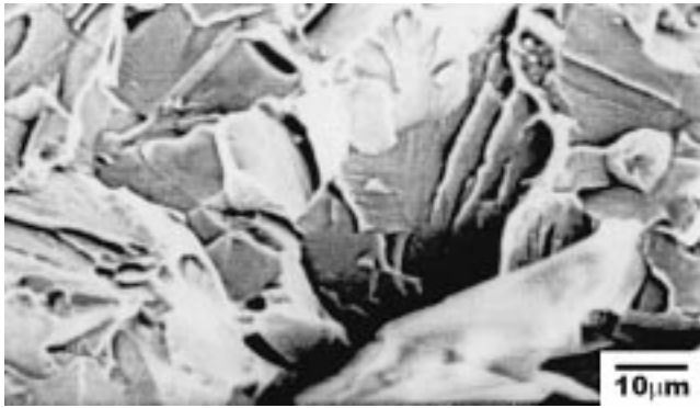
Fig. 23 Cleavage fracture morphology of a Charpy testpiece of the BM with an absorbed fracture energy of 20 J
