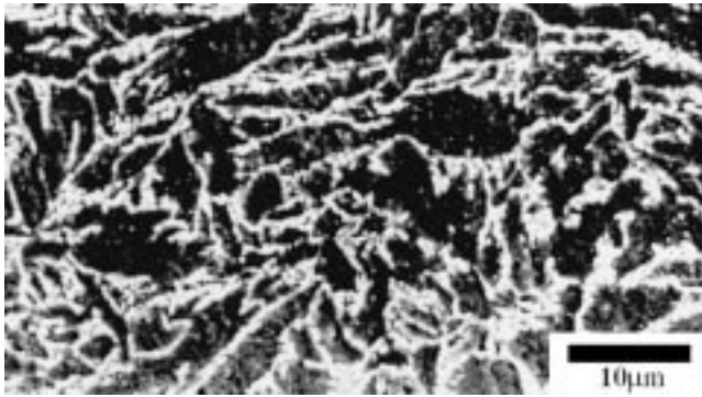
Fig. 9 Microstructure of the HAZ subjected to the heat treatment for 2.3 h. SEM
