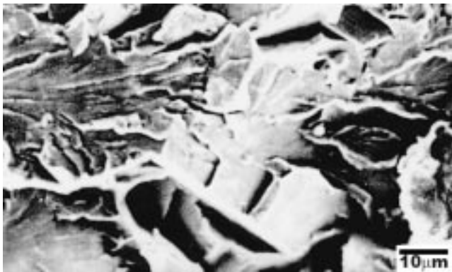
Fig. 24 Cleavage fracture morphology of a Charpy testpiece of the HAZ with an absorbed fracture energy of 20 J
